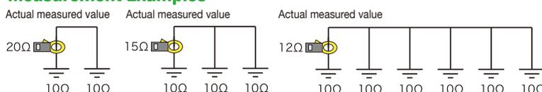
In multi-grounded system, the larger the number of grounding poles, the more accurate the measured value. Where the number of grounding poles are few, if just only one carries a very small resistance (e.g., 1Ω), the measured value will be close to the true value. On the other hand, poles with large resistances (e.g., 100Ω) will result in greater measurement uncertainties.
