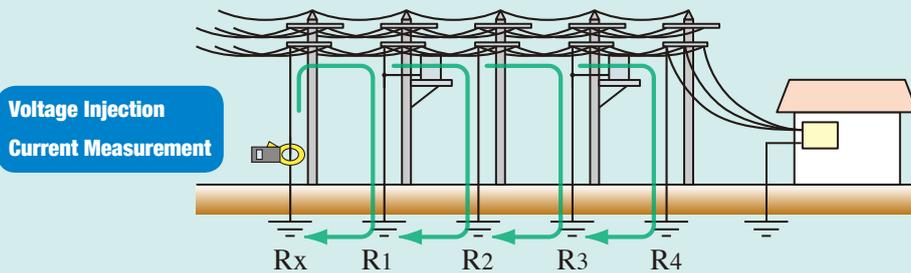
**Clamp on the earth cable. The instrument has two cores for voltage injection and current measurement.**
